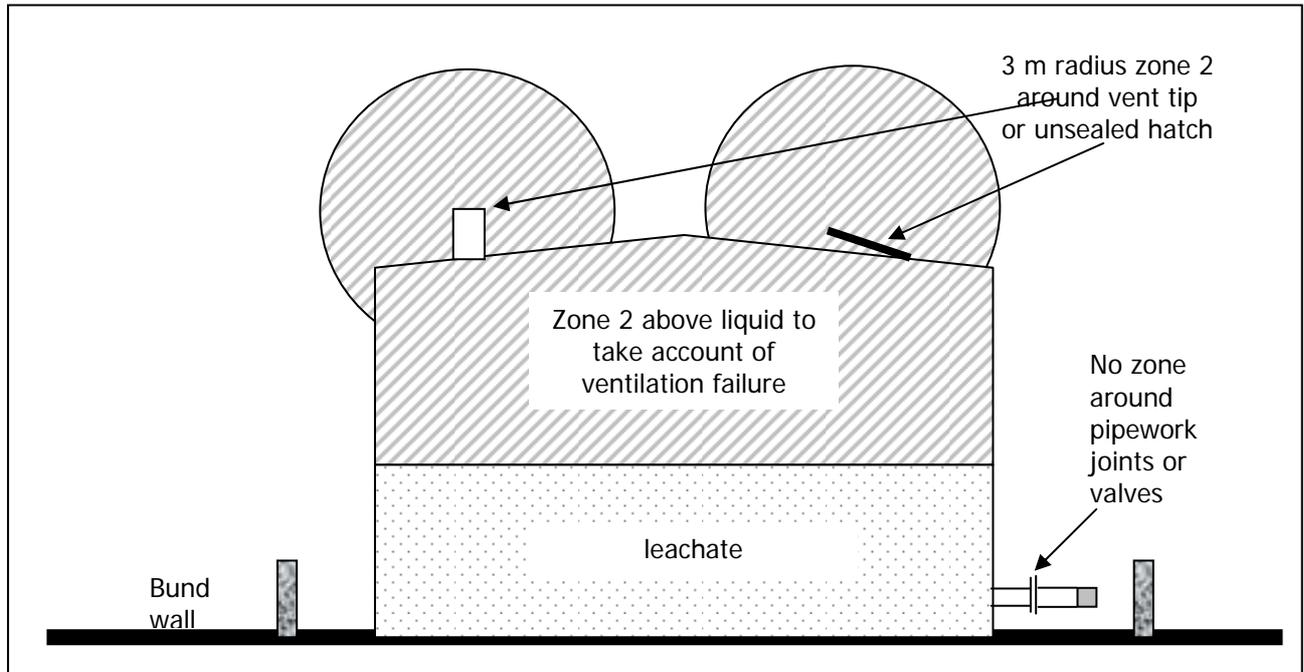
The zones 2 can only be changed to non-hazardous if standby ventilation automatically cuts in should the main ventilation fail.
