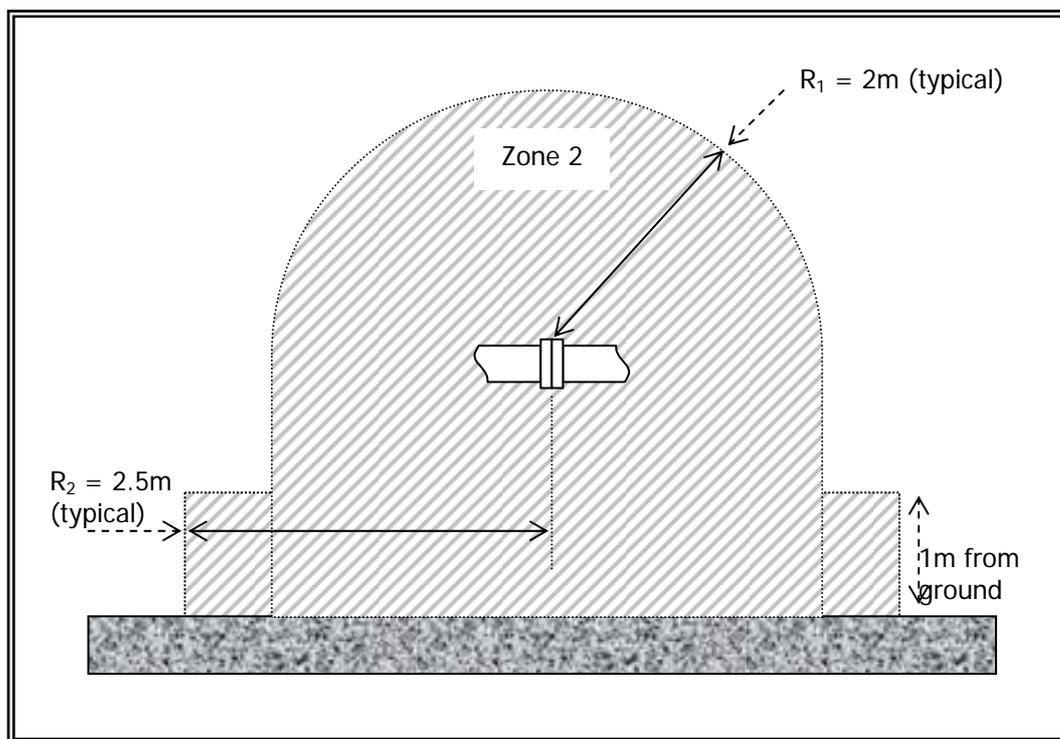
Many flanged joints give rise to smaller leaks than an equivalent hole diameter of 1 mm, depending on the integrity of the joint and whether operating conditions are adverse or relatively benign. IP15 Tables C9(a) and C9(b) do not give smaller values than those quoted above, so other methods can be used to define smaller zone extents if required; such methods are outside the scope of this ICoP.
