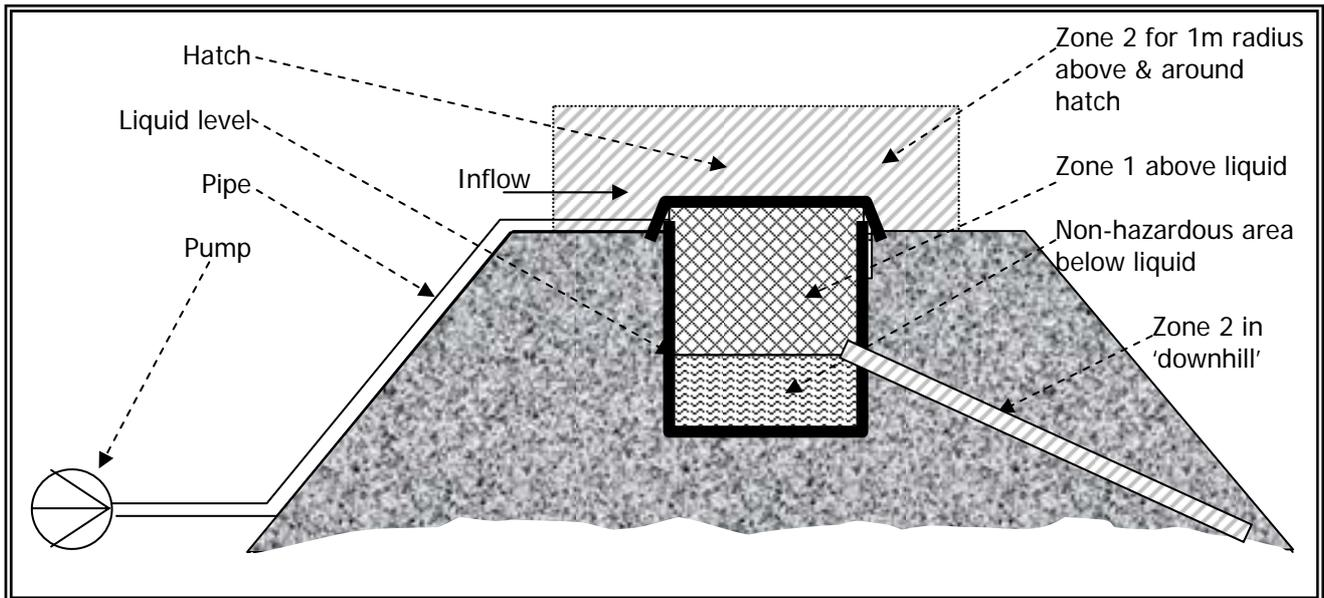
Break tanks that are used as collection tanks will have the same classification if there is an unventilated air space internally.
