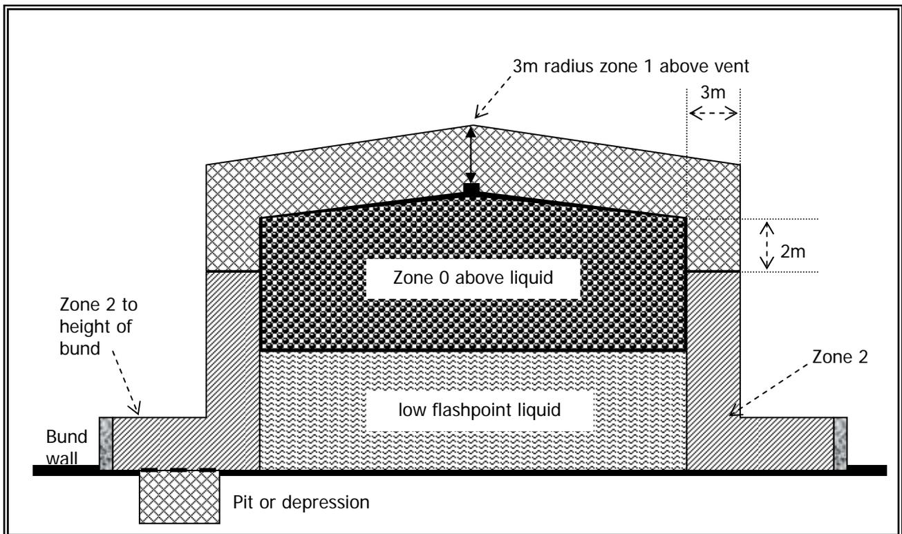
The zone 1 shown on figure 13 around the vent is due to vapour expelled when the tank is filled or gets warm. The zone 2 shown is in case of overfilling the tank or secondary grade releases in the bund, such as flanges and valves.<sup>36</sup>
