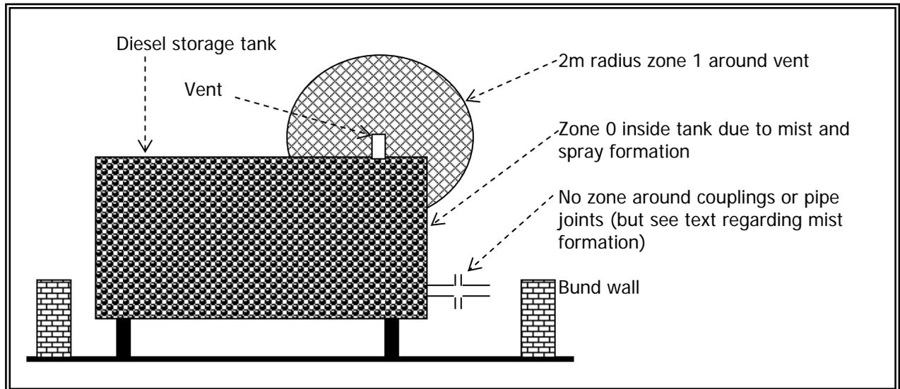
Diesel has a flashpoint of 55°C minimum, depending on the blend. IP15 clause A1.1 states: "To clarify the position pending further research, ....where a fluid is more than 5°C below its flashpoint and at atmospheric pressure or under only a few metres head in a storage tank, it can be treated as non-hazardous". Therefore diesel, which has a flashpoints more than 5°C above ambient, can be treated as non-hazardous provided it cannot leak onto a hot surface or be released as a mist.
