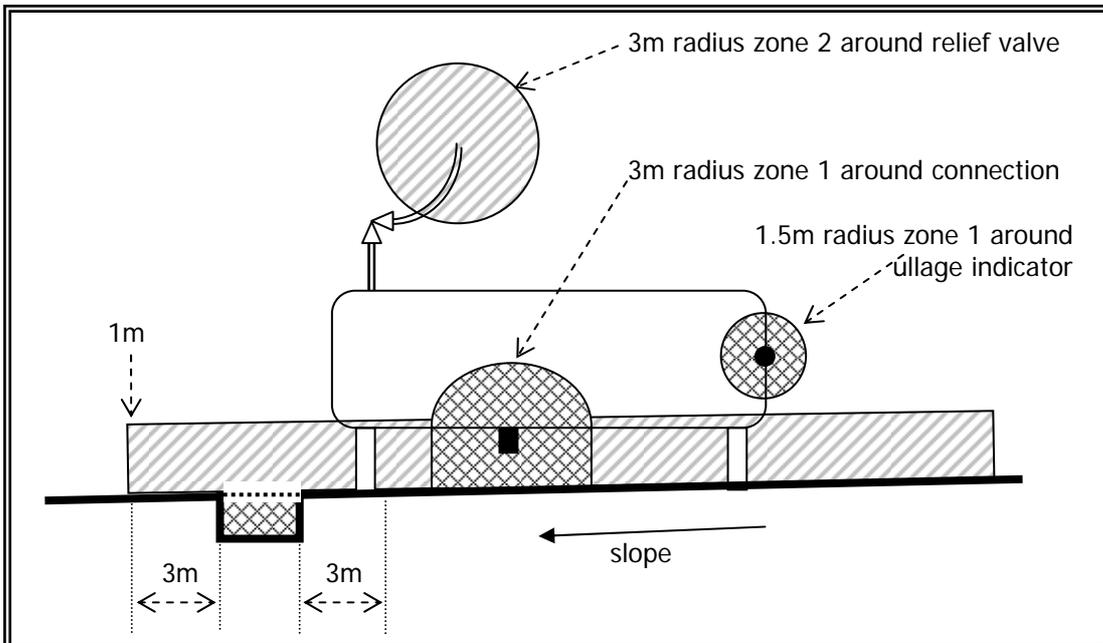
**Figure 9: zoning of a propane storage tank – plan view**
