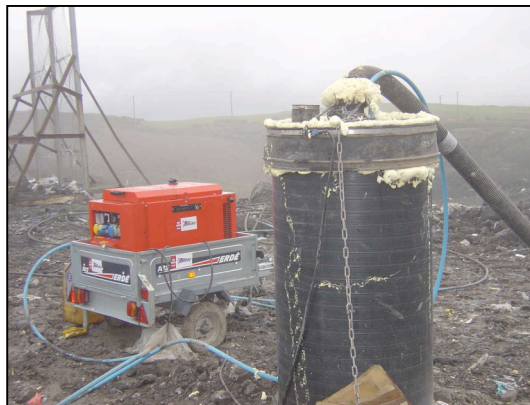
Photo 1: Generator located within a zone 2
