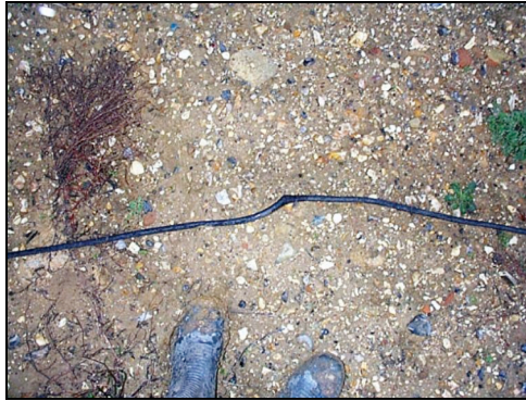
Photo 10: Badly repaired cable joint using electrical tape
