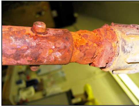
Photo 13: Lack of maintenance – excessive corrosion of borehole pump.
