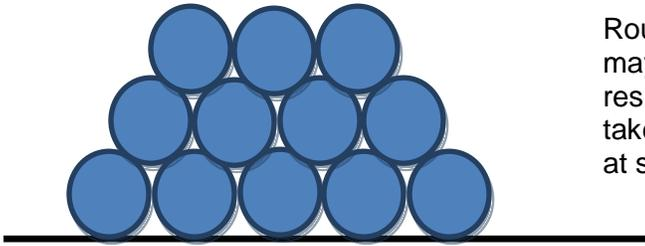
Round/tubular bales and loose materials which may roll should a stack collapse during a fire may result in fire spread – such factors need to be taken into account in your calculations to arrive at separation distances
