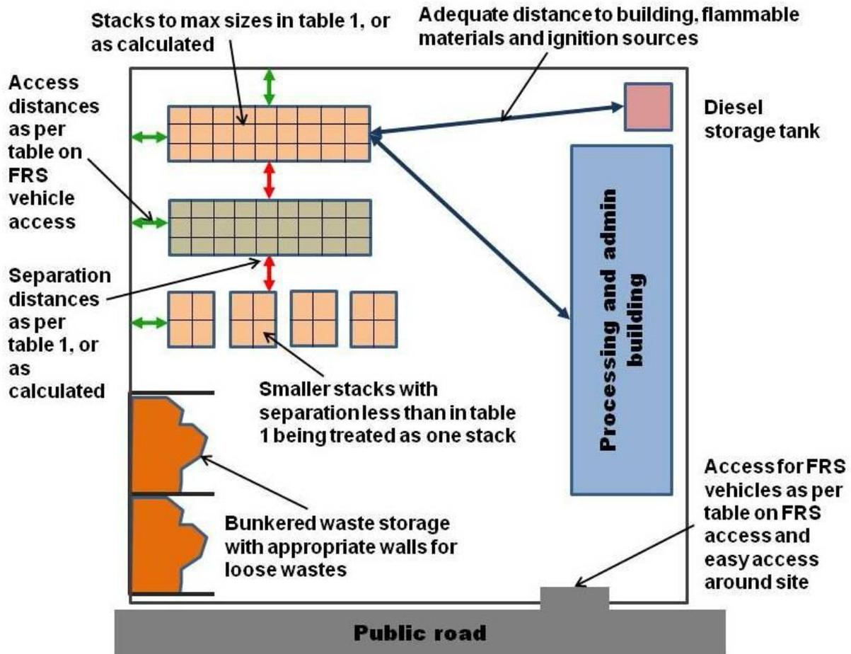
Note – the above example assumes that the site does not have residential or other buildings direct at its site boundary. If this is not the case then the distance between open stacks and boundary may be different to those simply set by FRS access requirements.
