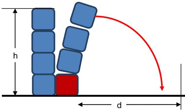
Assuming that the top bale will not roll significantly then a reasonable separation distance (d) would be at least 1 metre more than the height of the stack (h), given that the bale will split on impact with the ground. However, if the waste involved has significant elastic properties (such as tyres), there is the additional issue of the bale potentially bouncing.
