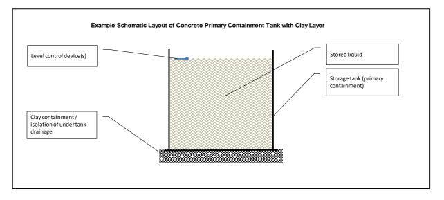
Example Tank Schematic ~ Concrete Tank with Clay Under-layer
