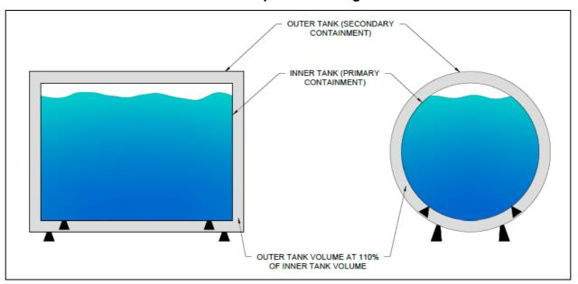
These are both acceptable as long as they are supplied from reputable suppliers and conform to the design elements laid out in Section 6.0, 7.0 and 8.0). The need to protect such tanks from credible impact scenarios is highlighted as they are more susceptible to complete failure from such damage than other engineered tank and bund designs.
