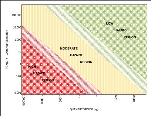
**Source Hazard Determination Diagram**
