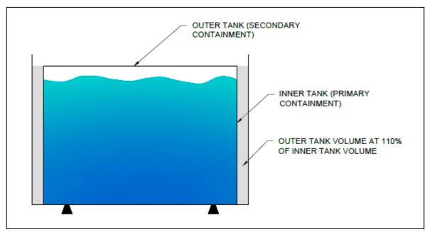
Figure 2 'Double Skinned' Tank
