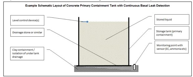
Example Tank Schematic ~ Concrete Tank with Engineered Clay Isolation Layer and Leak Detection
