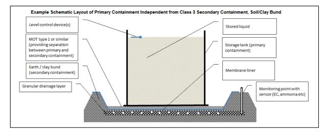
Similar leakage detection systems would need to be employed where buried or part buried tanks were required.
