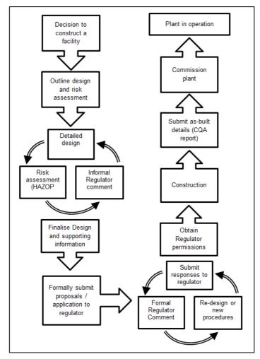
Figure 1 Simplified Project Steps Flow Diagram
